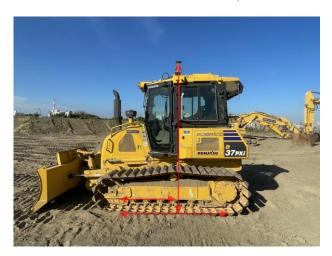
\* Measure on as a flat place as possible. The height may not be measured correctly on a slope.
