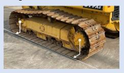
The measurement of the last fifth point is to recognize the right side of the machine body. Measure the ground contact surface near the right side of the machine body. Refer to the tablet screen.
