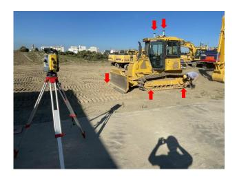
\* Set the TS at a position enabling measurement of the left side of the machine body, as shown on the tablet screen.
