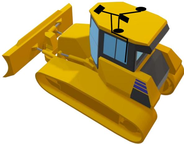
IMU connector faces left side of vehicle body
