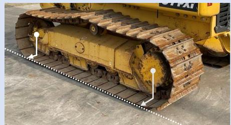
The measurement of the last fifth point is to recognize the right side of the machine body. Measure the ground contact surface near the right side of the machine body. Refer to the tablet screen.
