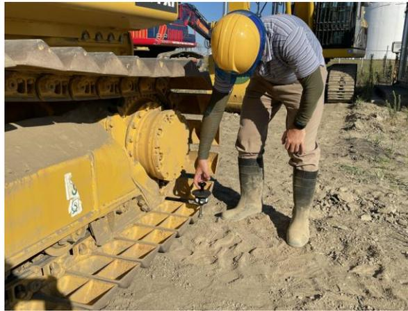
4. Similarly, input the measurement result of the ground contact point on the front left side of the machine body on the tablet screen.
